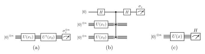
Fig. 1 Fig. 1(a)-(b) Fidelity test and SWAP test for Quantum Kernel Estimation where U is the feature map associated with the quantum kernel. Figure 1(c) Quantum circuit for the feature map associated with the projected kernel, the Hermitian observable H can be arbitrary
