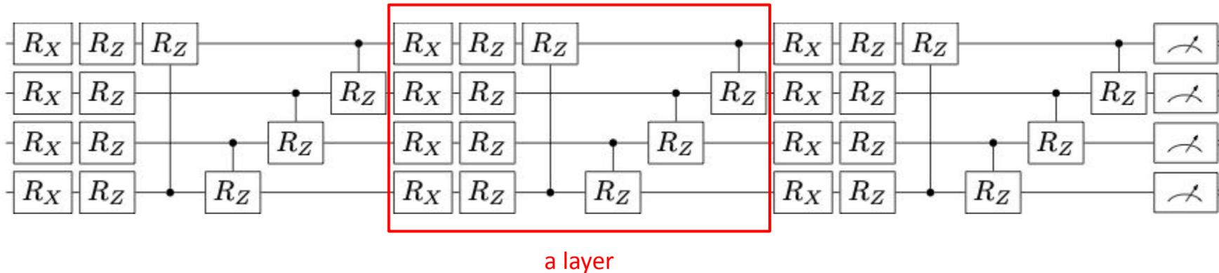
Layers are repeated blocks of Quantum Circuits.
